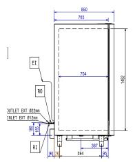
Drain Electrical inlet (power) RO Refrigerant Outlet
